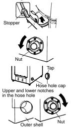
5 Turn the stopper 180° without removing from hose. Insert the stopper into the securing hole on the left side of the outer shell and press down to secure the internal hose.
